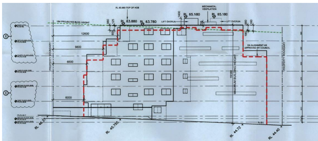
Figure 3: Eastern elevation indicating the building height breach is predominantly isolated to the northern portion of the development and the lift overrun. The green line indicates the 18m building height limit. The red line indicates the originally approved development.
