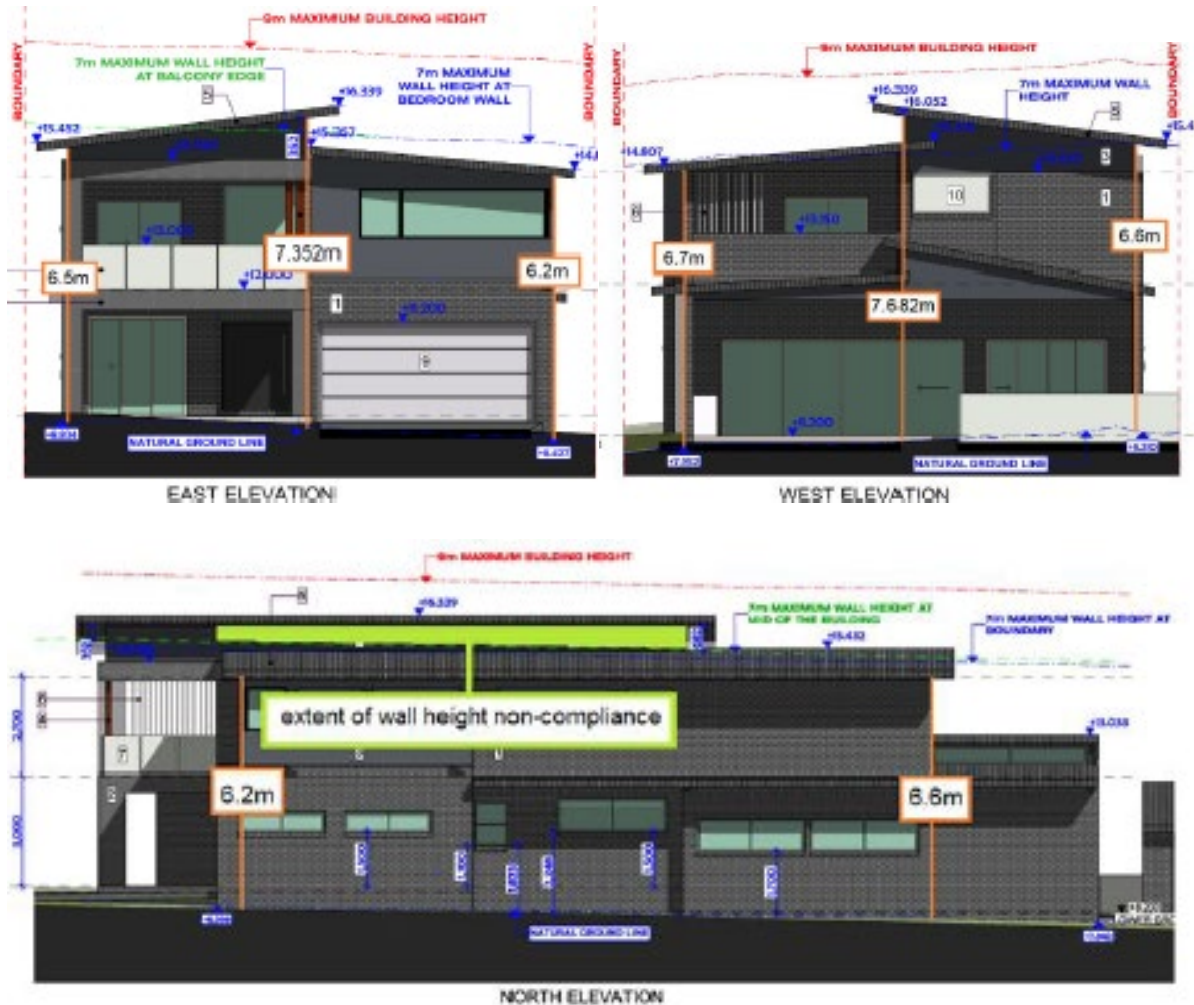
Figure 3: East, West and North Elevation identifying Extent of Wall Height Non-compliance
