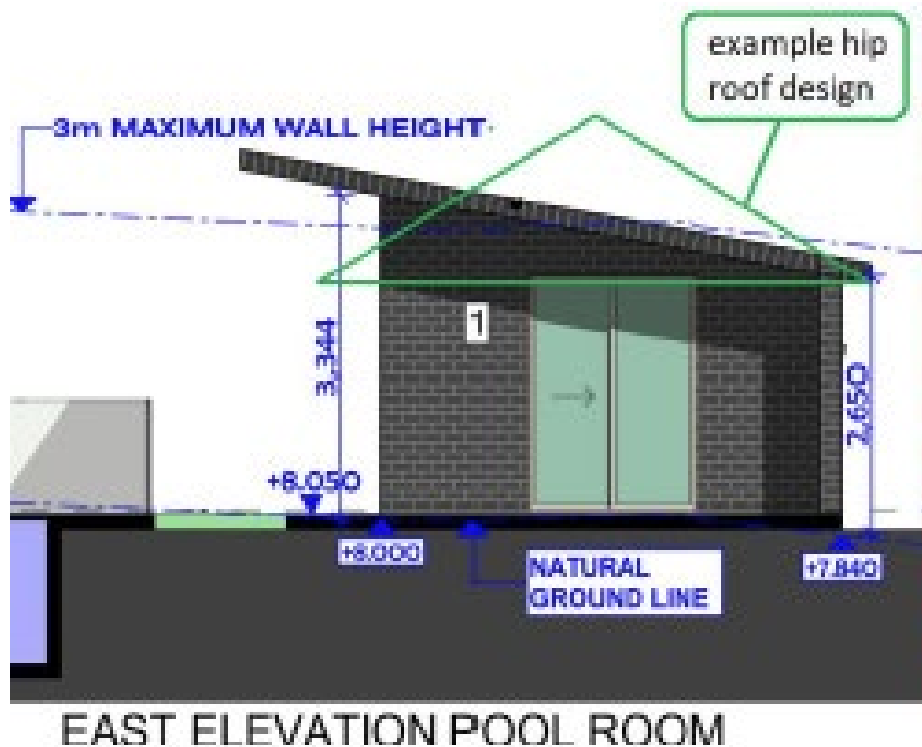
Figure 4: East Elevation of Outbuilding / Pool Room identifying Extent of Wall Height Non-compliance
