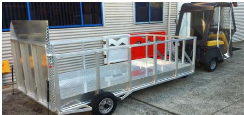
Figure 18: Aluminium Trailer attached to an Electric Tug Device
