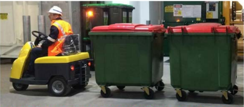
Figure 16: Universal Towing Device pulling 1100L bins behind an Electric Tug Device
